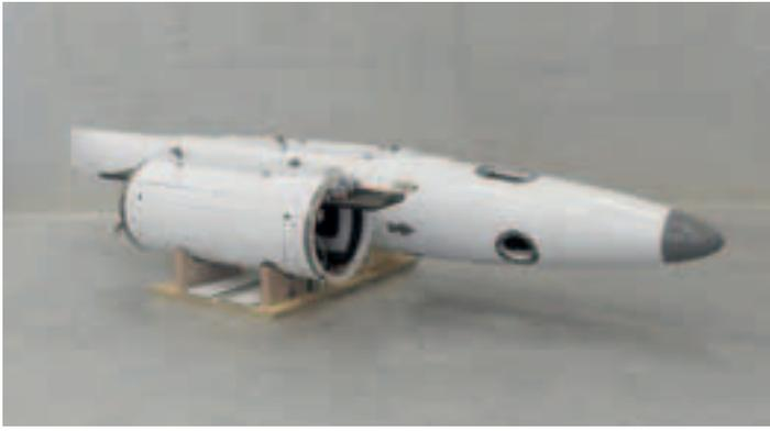
**CFRP in action: Instrument carriers and complete underwing pod for the research aircraft HALO, developed and manufactured by Aerostruktur**
