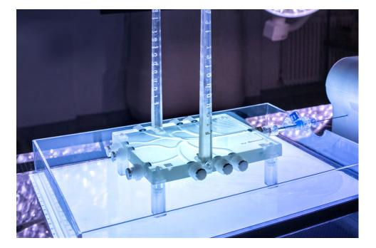
**Printed vessel phantom with guide wire for a catheter.** Source: Fraunhofer IPA; photo: Vanessa Stachel
