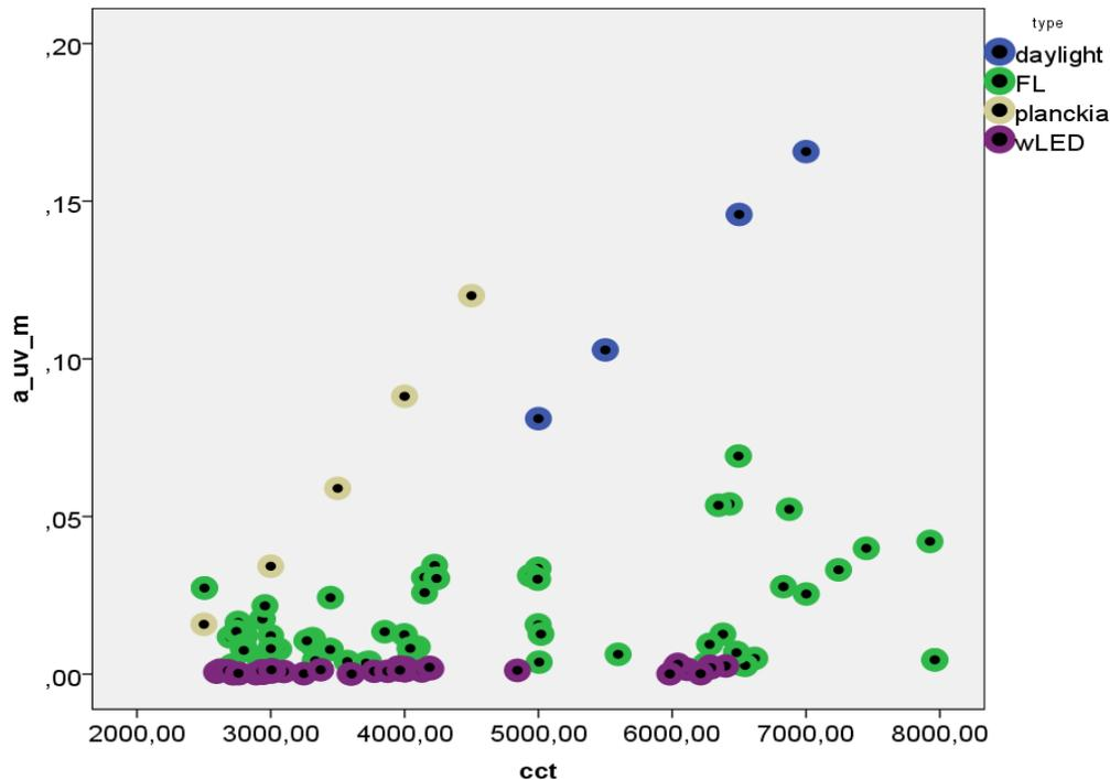
Figure 3. Relative spectral content of radiation in Monico et al.’s “UV window” ( $a_{uv,m}$ ) for each one of the 118 light sources grouped by the type of light source, white LED (wLED), fluorescent lamp (FL), daylight and Planckian radiator, as a function of correlated colour temperature (CCT)
