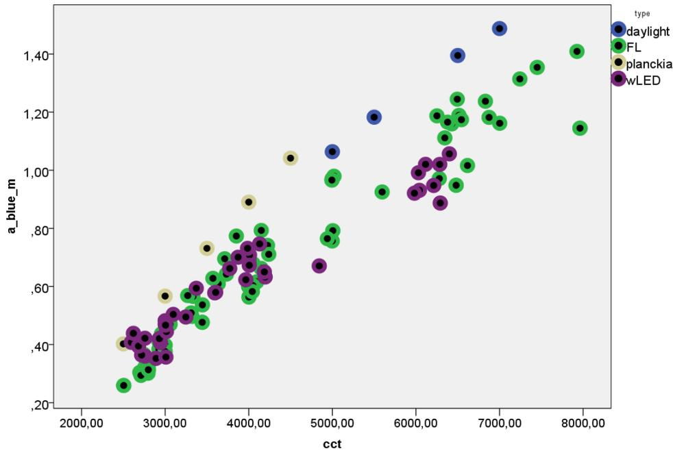
Figure 2. Relative spectral content of radiation in Monico et al.’s “blue window” (**a\_blue\_m**) for each one of the 118 light sources grouped by the type of light source, white LED (wLED), fluorescent lamp (FL), daylight and Planckian radiator, as a function of correlated colour temperature (CCT)
