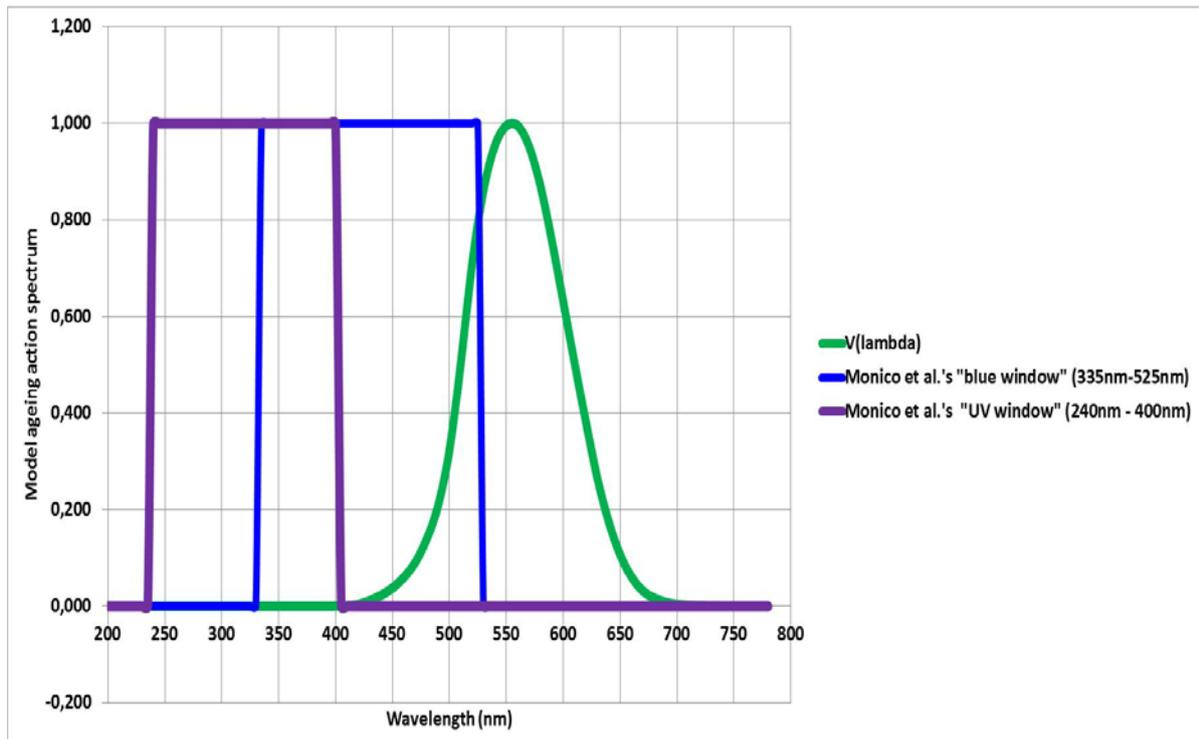
Figure 1. Monico et al.'s two spectral ranges or “spectral windows” (UV and blue) compared to the photopic luminous efficiency function  $V(\lambda)$
