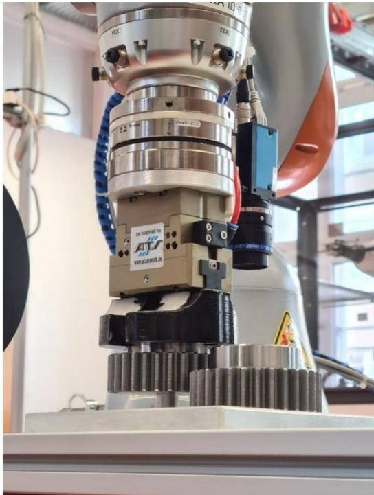
**Fig. 1 Robotics can be that simple and efficient: controlled by 2D images, the robot picks up a component and, thanks to intelligent AI, fits it into a second gear using force/moment control. Munich University of Applied Sciences, March 22, 2024**
