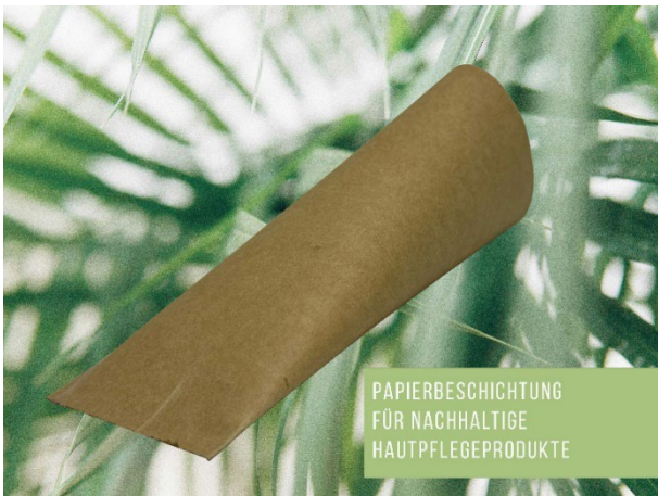
Fig. 2 Coated paper with a barrier effect for the production of cosmetic tubes. In addition to the Fraunhofer ISC, the project partners Polymaris, IPC and Albea were involved in this project.
