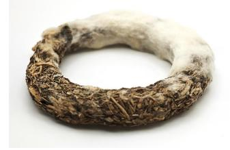
Abb. 2 Depending on the composition of the substrate, type of fungus, and growth conditions, various properties of fungal mycelium-based materials can be deliberately adjusted during cultivation, such as hard and solid structures © Fraunhofer IWU www.iwu.fraunhofer.de
