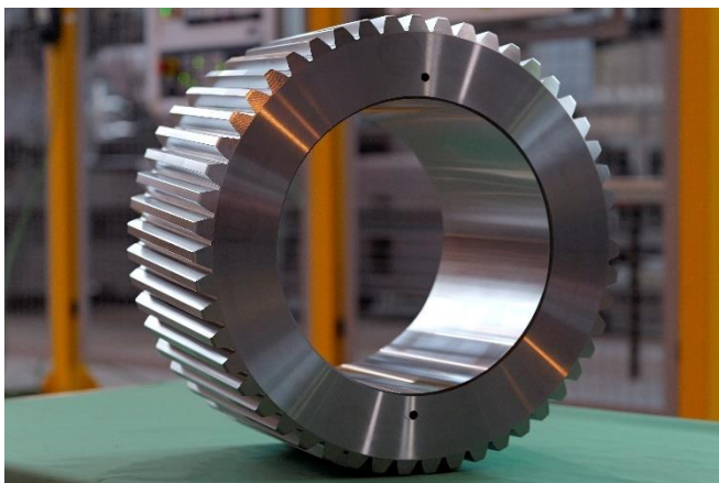
Fig. 2 Damaged transmissions in offshore wind turbines require expensive repair work – using highly durable gears like those developed in GEARFORM pays off
