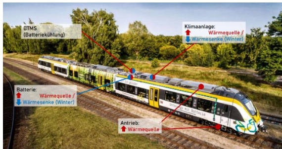
Fig. 1 The drive system, passenger compartment, and—depending on the propulsion system—the energy storage of a train always requires an ideal temperature range. The air conditioning system and battery are heat sinks in winter, otherwise they are heat sources. The drive system is a heat source year-round.
