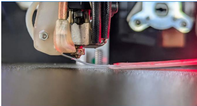
Fig. 4 The FEAM process uses fiber material made of glass, which is applied to any substrate via a polymer coating without affecting its optical properties. © Fraunhofer IWU
