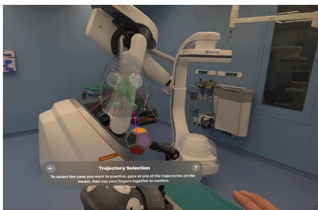
Fig. 3 Field of view of the surgeon: The actual operating room is visible in the glasses. The app "places" individual patient data on the actual head. First, the surgeon selects the access path (trajectory) to the operation site. The fully automatic registration (calibration, real-time recognition of the surgical instrument) takes just one second. © Fraunhofer IWU
