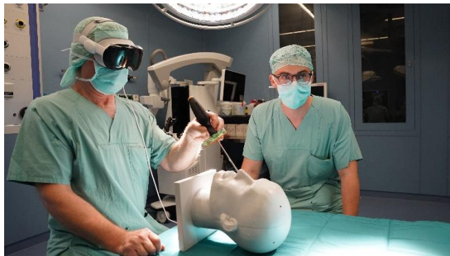
Fig. 1 Neurosurgeon Prof. Dr. Dirk Winkler and computer scientist Conrad Günther (UKL) test the app for neurosurgical spatial navigation on a model head. Thanks to the real and virtual information visualized in standard data glasses ("Mixed-Reality"), the operating surgeon can safely guide his instrument and minimize the risk of causing injuries. © Fraunhofer IWU
