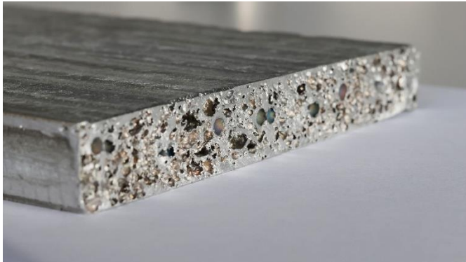
Fig. 1 The composite material HoverLIGHT has a core made of aluminum foam with encapsulated hollow spheres (visible in the cross-section as round openings). The combined damping effects of foam and particle-filled hollow spheres are comparable to those of magnesium. © Fraunhofer IWU
