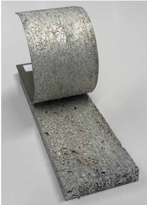
Fig. 3 Sticks: The drum peel test (DIN 53 295) proves that the cover sheets and sandwich core form a stable bond. © Fraunhofer IWU
