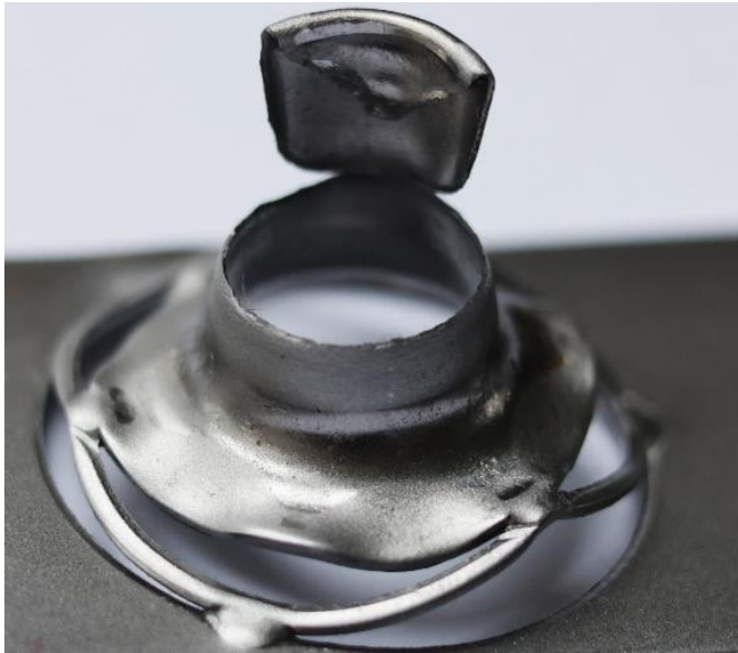
Fig. 2: With identical parameters but without ultrasonic support, the metal cracks.
