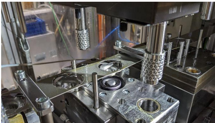
Fig. 3: Series-capable: Deep drawing with ultrasonic actuation under the die.
