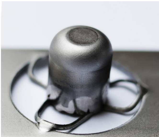
Fig. 1: Ultrasonic deep drawing makes the difference: with a drawing ratio of 2.3 and vibration support, the deep-drawn bowl.
