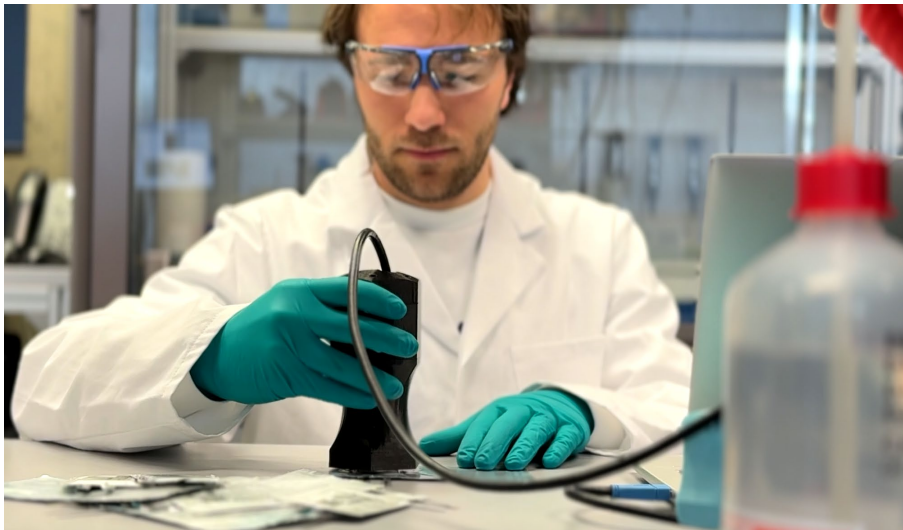
Easy reading of information from battery cells marked with fluorescent markers © K. Selsam, Fraunhofer ISC / IDcycLIB
