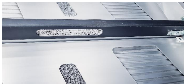
Fig. 2 Aluminum foam sandwich structure.
