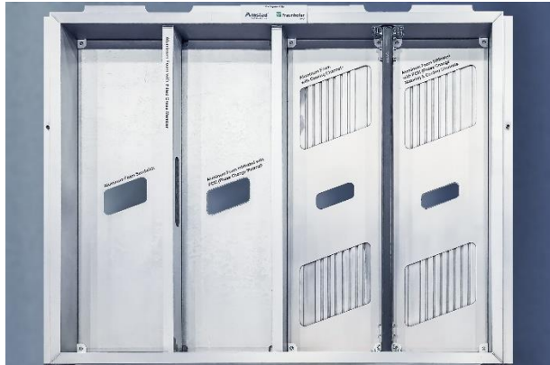
Fig. 1 Options for housing structures. From left to right in the four chambers: pure AAS, AAS with infiltrated PCM, AAS with cooling structure, and AAS with cooling structure and PCM.
