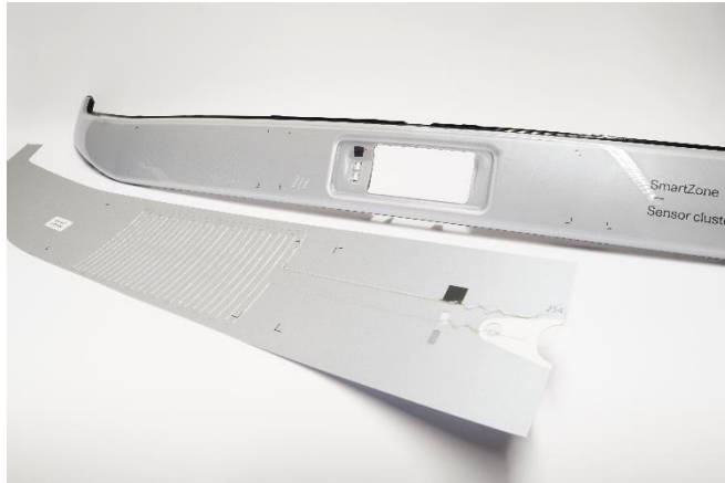
Fig. 2 Highly flexible, stretchable, and 3D-formable PCBs – WEAM printing of a 0.1 mm diameter copper trace on a 0.1 mm thin thermoplastic polyurethane film © Fraunhofer IWU
