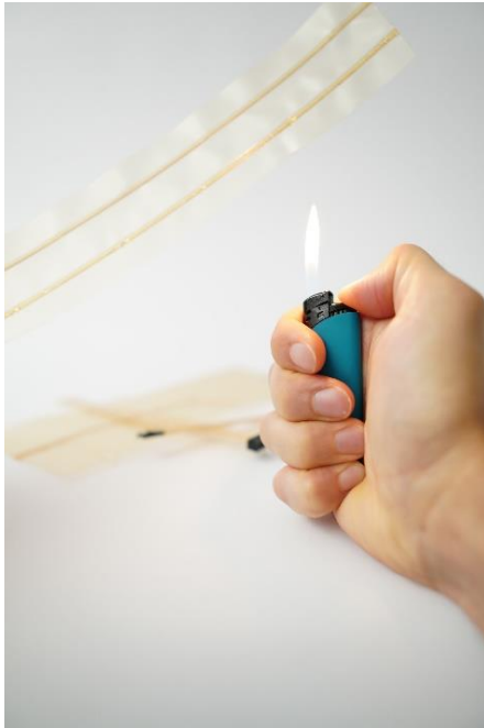
Fig. 3 PFAS-free high-temperature flexible conductors © Fraunhofer IWU
