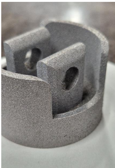
Fig. 4 Aluminum Matrix Composites combine low density with excellent wear resistance. © Fraunhofer IWU
