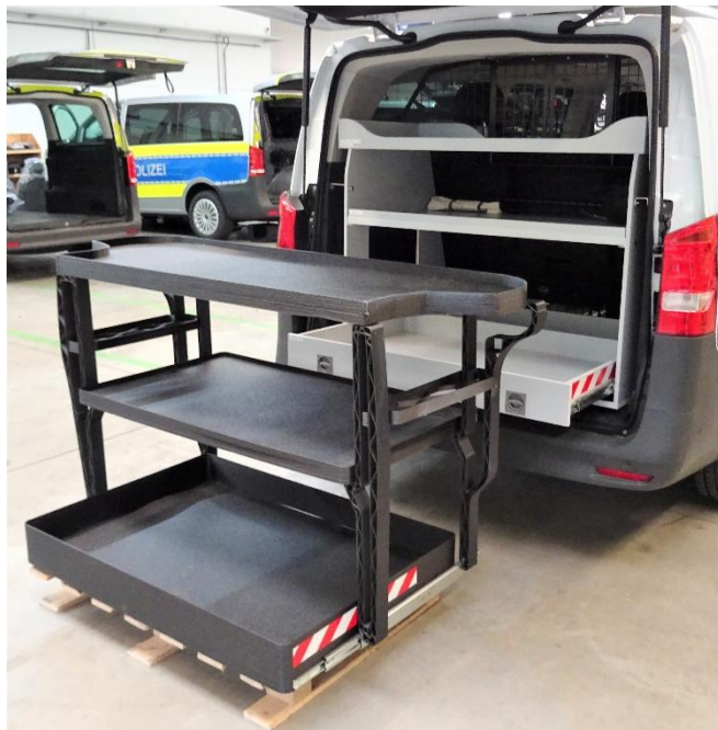
Fig. 2 Fraunhofer IWU and MOSOLF Special Vehicles GmbH have developed a 3D-printed rear shelf for the Mercedes Vito, saving 26.5 kg compared to the previous retrofit solution, including the hardware. The printed shelf fits perfectly into the vehicle body, requiring no additional reinforcements or fasteners, and optimally utilizes space in the rear. © MOSOLF Special Vehicles GmbH
