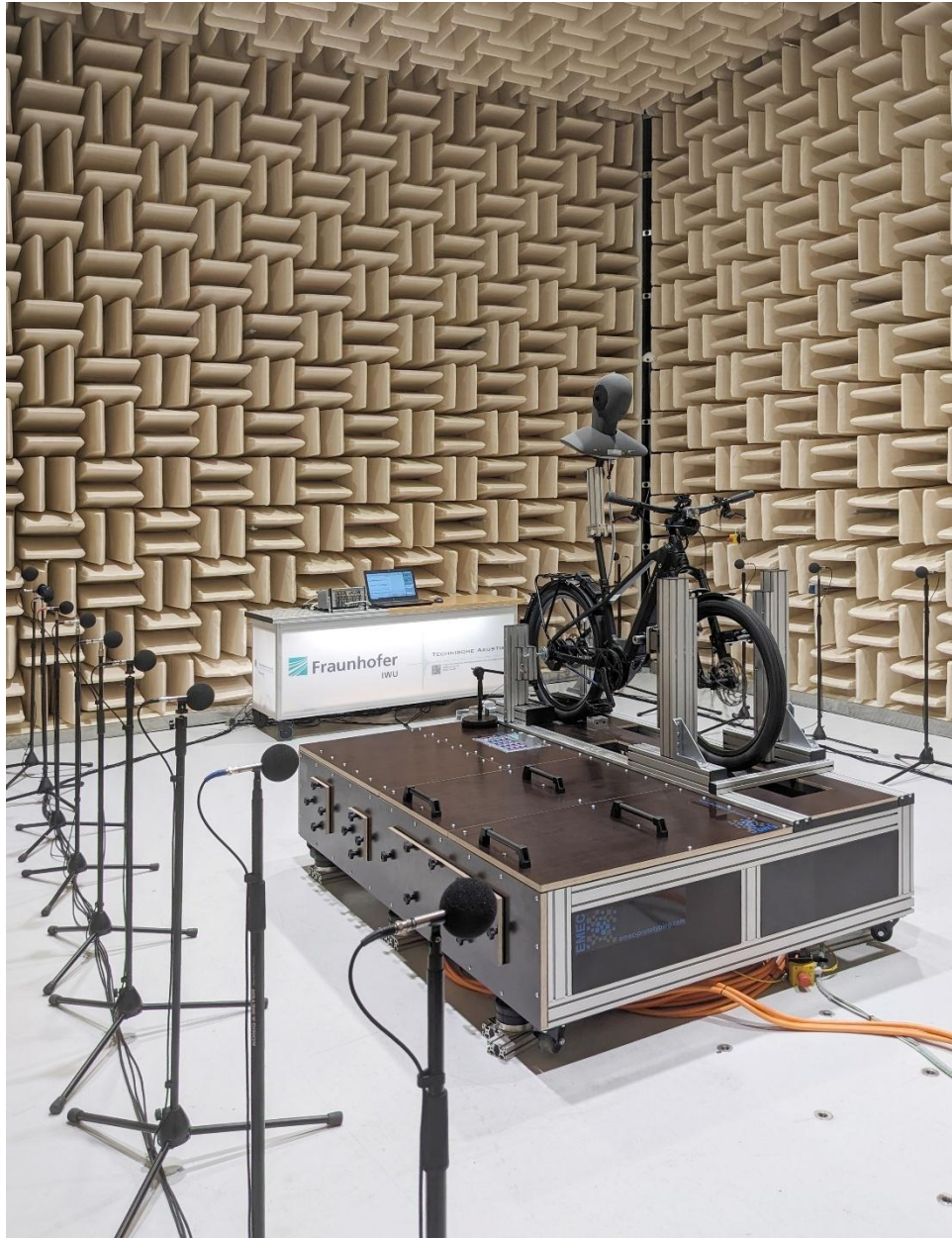
Fig. 1 The acoustic test rig, developed by EMEC Prototyping GmbH and validated jointly with Fraunhofer IWU, during tests with a high-end e-bike at Fraunhofer IWU Dresden. © Fraunhofer IWU
