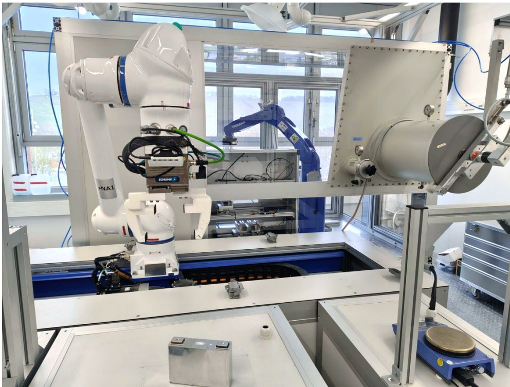
Roboter device for automated disassembly of batteries for ReUse at Fraunhofer ISC © Fraunhofer ISC
