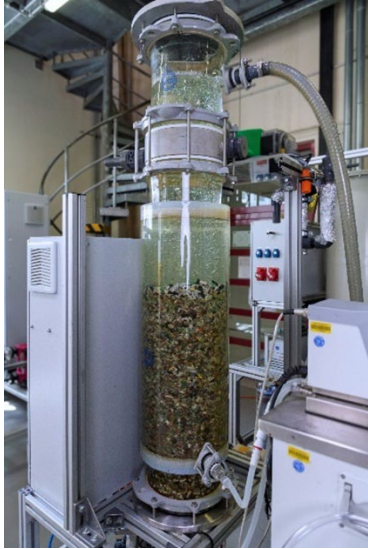
Figure 2 Fraunhofer IGB has developed a fixed-bed circulation reactor for recovering materials such as rare earths from electronic waste.
