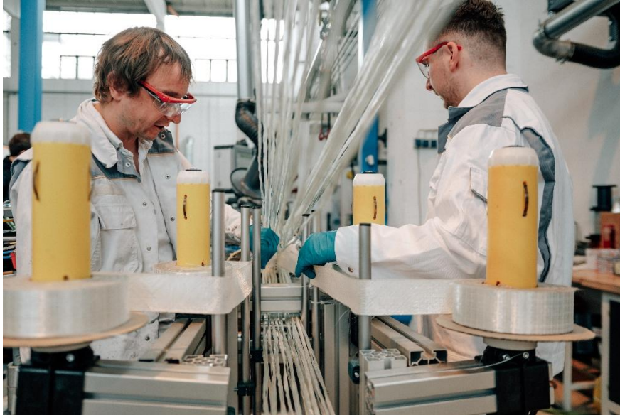
Fig. 1 Pultrusion: long, lightweight, and high-strength composite profiles. © Fraunhofer IWU
