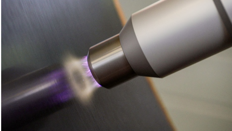
Figure 1 | Caption "HYTANK" – Contactless atmospheric-pressure plasma pre-treatment of a CFRP surface (© Fraunhofer IFAM).
