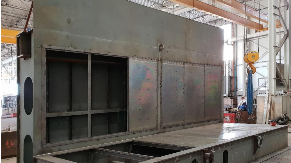
Fig. 3: Prototype cargo hold section (one half) for an inland container vessel. The sandwich panels used measure 2 m × 1 m and have thicknesses ranging from 14 mm to 28 mm.
