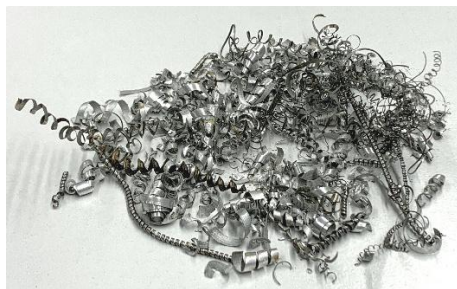
Fig.2 Aluminum alloy chips as a feedstock for high-performance lightweight construction materials. © Fraunhofer IWU
