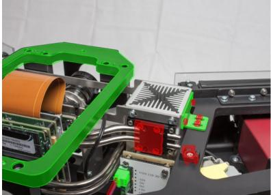
In model-based assembly inspection, software compares the digital target data of assembled components with the real outcome. Errors are detected
