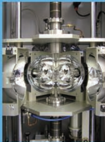
Ultra-high vacuum compatible image furnace for the growth of single crystals. (TUM)
