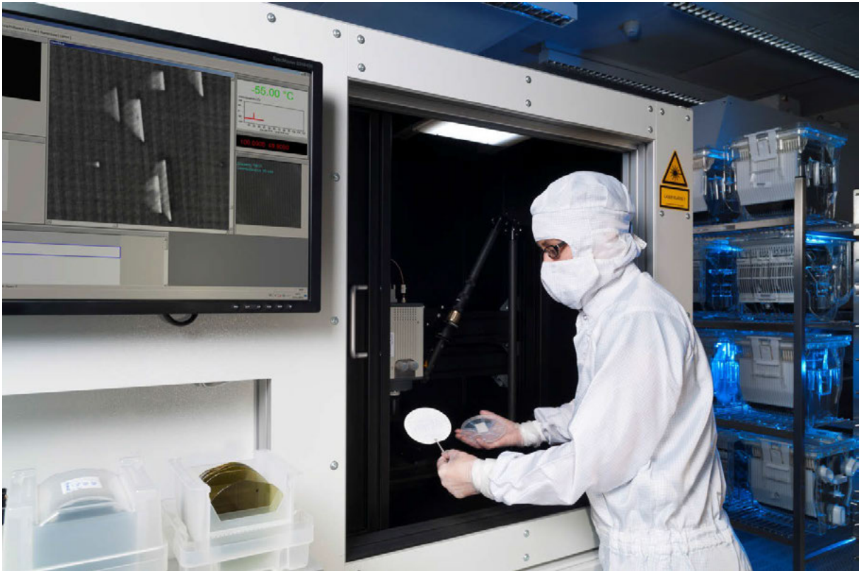
Figure 1: Operator loading a 100 mm SiC epiwafer in the defect luminescence scanner at Fraunhofer IISB. © Fraunhofer IISB
