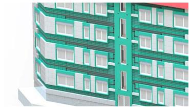
Model shows the wiring and pipes integrated in the façade of a demonstration building from the 1950s in Frankfurt, Germany. ©Fraunhofer ISE
