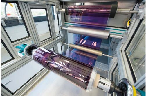
Electrochromic coating, applied under clean room conditions on the new roll-to-roll coating plant
