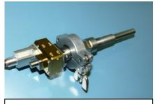
The CTR research centre's laser ignition system will be integrated in a combustion chamber for cryogenic fuels and rendered fit for space. © CTR
