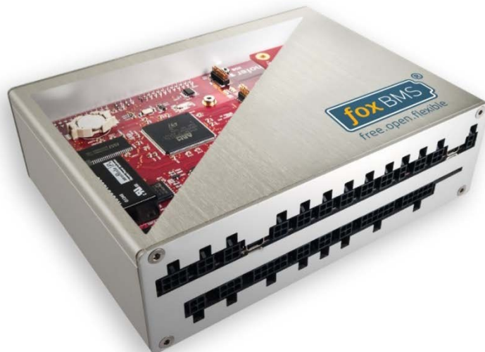
Central control unit of foxBMS, the free, open, and flexible battery management system from Fraunhofer IISB in Erlangen. Picture: Fraunhofer IISB
