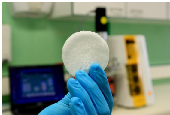
Fig. 2: Wound dressing (nonwoven/fleece) made from alginate fibres derived from bacteria. Bacterial alginate nonwoven materials absorb up to 70% more liquid than marine alginate nonwovens.
