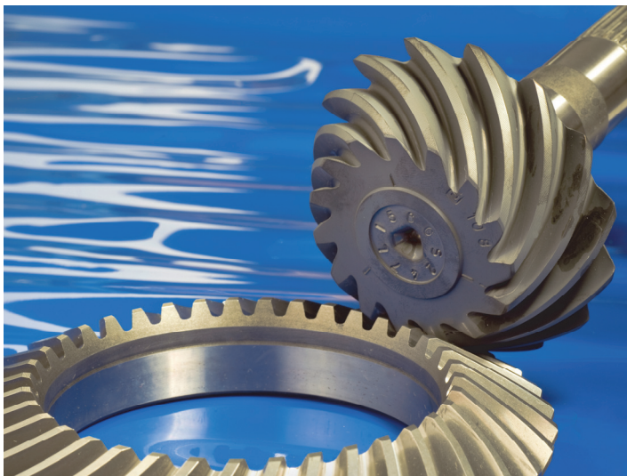
Coating of gear components with super hard Diamor® films by means of laser-arc technology © Frank Höhler
