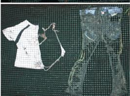
Biodegradation of textiles The start, the third excavation after seven weeks and the last digging after 14 weeks in an earth burial test in which the degradability of the materials is assessed. The textiles are put on a grid and placed in the burial position. The left side of the t-shirt is 100% polyester and the right side is 100% cotton. The jeans are 99% cotton and 1% elastane. They are buried in microbiologically standardised earth. © Hohenstein Institute
