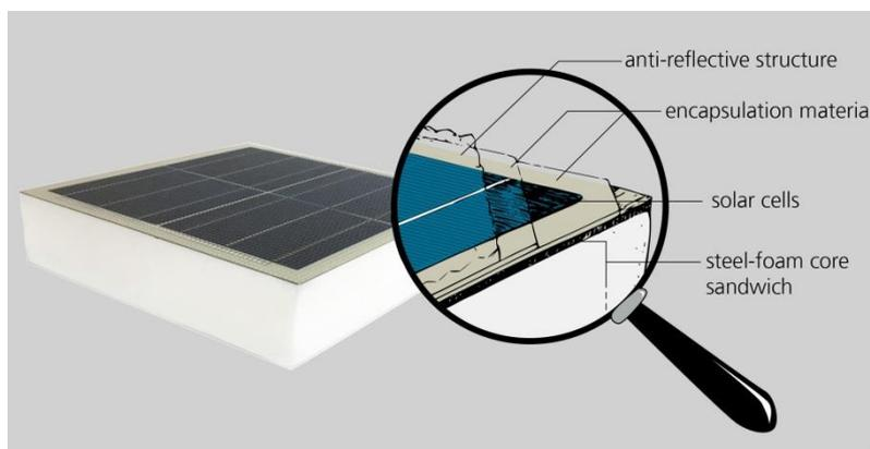
Principle of the vehicle-integrated PV modules for refrigerated semitrailers developed by Fraunhofer ISE.
