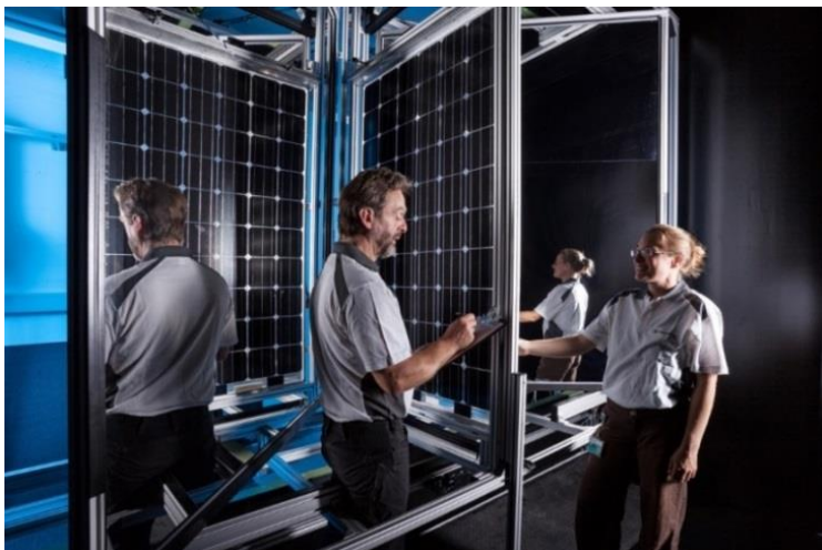
Test stand developed at Fraunhofer ISE for measuring bifacial PV modules. ©Fraunhofer ISE
