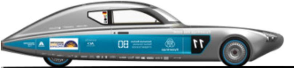
thyssenkrupp blue.cruiser: 117 kg CFRP
