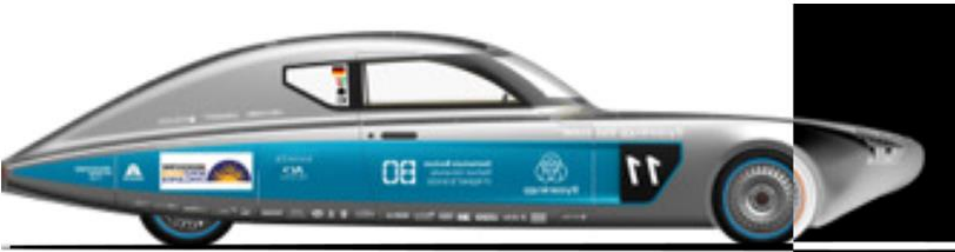
thyssenkrupp blue.cruiser: 111kg CFRP, 12 kg NFRP
