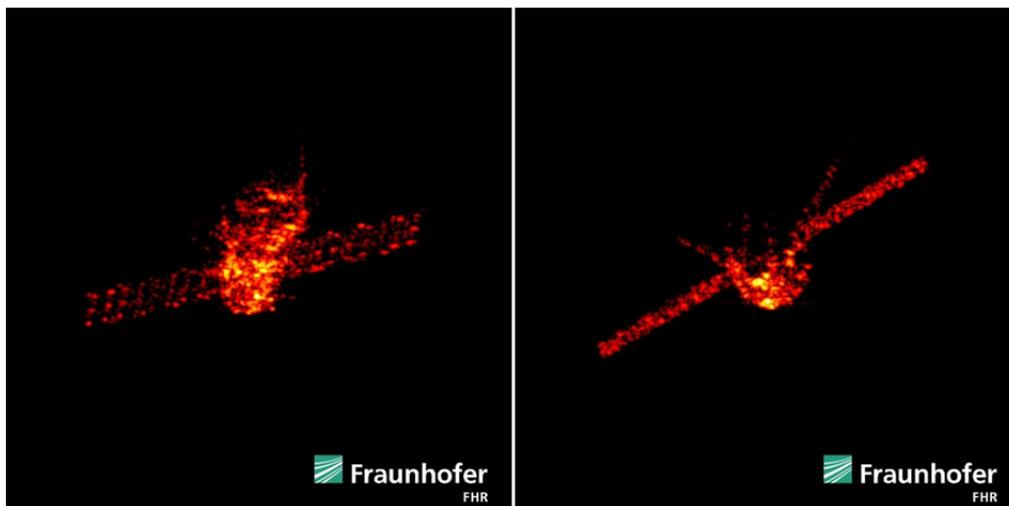
Radar images of Tiangong-1 from different perspectives taken at an orbital height of approx. 270 km above the Earth's surface. The main body and the solar panels of the space station are clearly visible.
