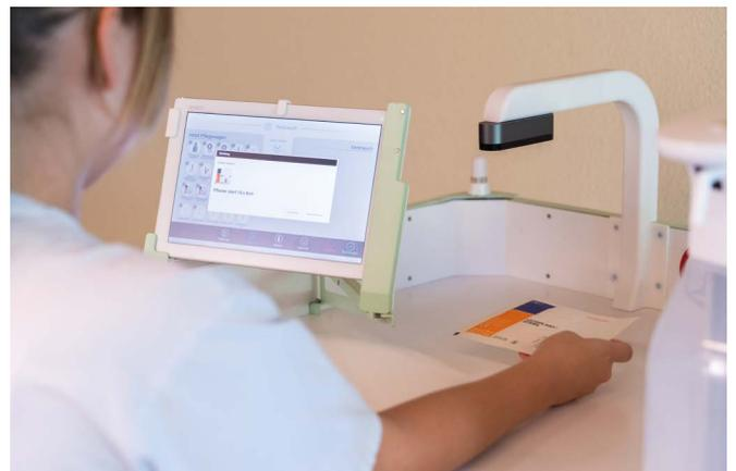
**Figure 3 Intelligent care cart:** The 3D sensor detects which item was removed. The nurse confirms this on the tablet, which dispenses with the need to keep manual records.
