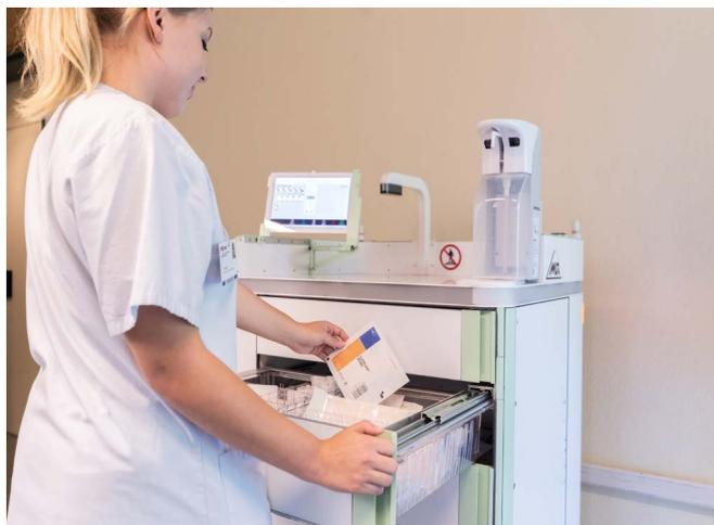
**Figure 2 Intelligent care cart:** The care cart is of modular design and can be adapted to different application environments, such as care homes or hospitals. The drawers are locked until a member of the nursing staff logs on.
