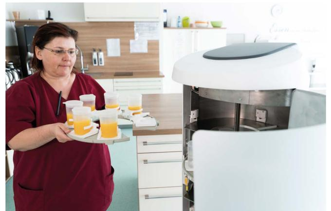
**Figure 3 Robotic service assistant** The service assistant can hold up to 28 cups or various snacks. Once they have all been served, the robot returns to the kitchen, where it is restocked by the staff before being sent back to the day room by the use of a smartphone.
