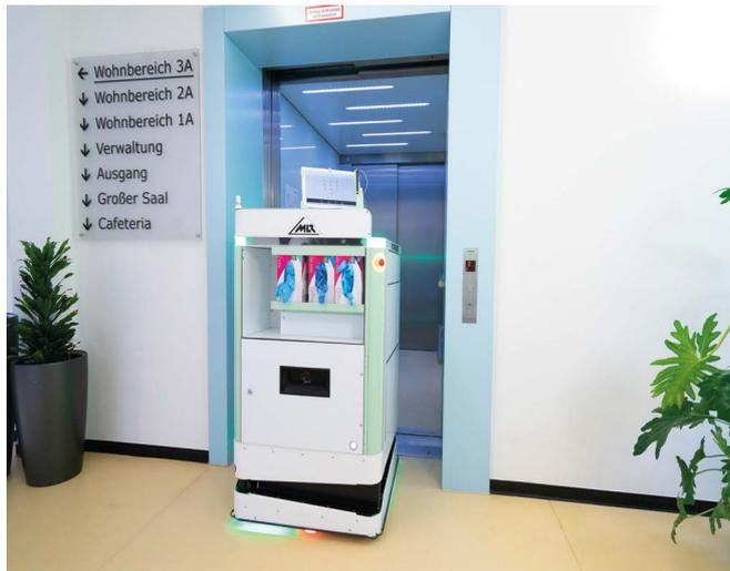
**Figure 1 Intelligent care cart:** The intelligent care cart makes its own way to the desired room and is also capable of using a lift. It can be summoned by the nurse from a smartphone, which means less legwork for staff.
