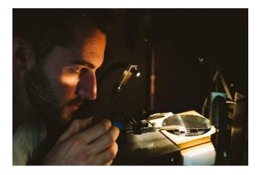
With the tandem solar cell made of silicon and III-V semiconductor materials, a more energetically efficient use of the solar spectrum is possible, compared to conventional solar cells available today. ©Fraunhofer ISE/ A. Wekkeli
