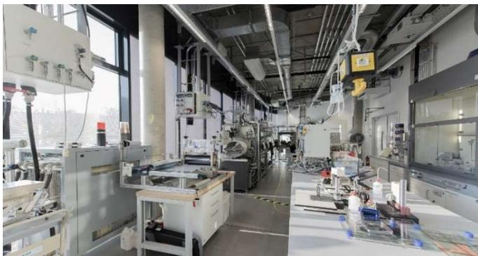
At the Fraunhofer ISC, Würzburg, the complete process chain for the production of battery cells is available. Currently, the area for assembly under protective gas atmosphere is being further expanded (in the picture at the back left). Picture: K. Selsam, Fraunhofer ISC
