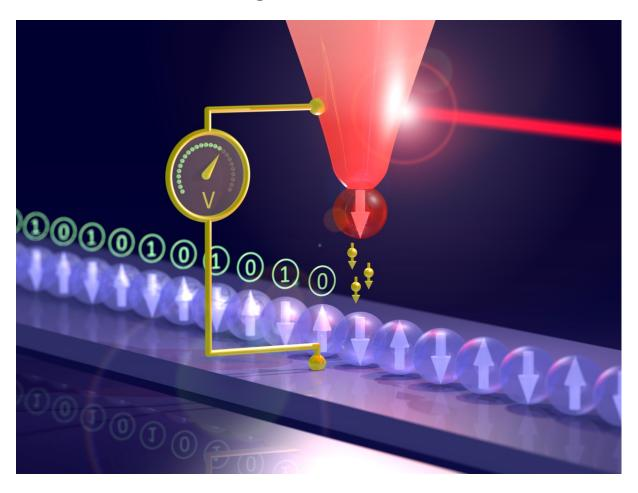
The illustration schematically depicts the experimental setup: The tip of the scanning tunneling microscope is heated using a laser beam. The temperature difference between the hot tip (red) and the cold surface atoms (blue) generates an electric voltage (yellow), which depends on the magnetic orientation of the surface atoms, acting here as magnetic bits (green). (Image: UHH/Krause)
