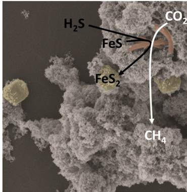
Electron microscopy image of a pyrite forming culture enriched from a wastewater treatment plant. Microbial cells are highlighted in red and pyrite crystals in yellow. The interdependency of pyrite ( $\text{FeS}_2$ ) and methane ( $\text{CH}_4$ ) formation is illustrated schematically.
