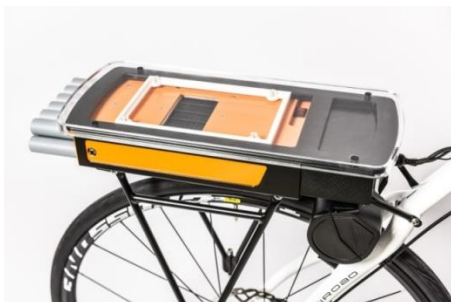
The electric bicycle rack with fuel cell only weighs 3.3 kg including hydrogen tank. It can be mounted on any bike. © Fraunhofer ISE
