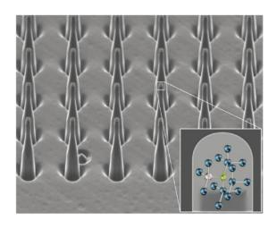
Structured monocrystalline diamond tip. Inset: atomic structure of an NV center in diamond.
