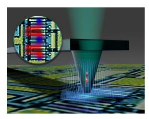
Schematic visualization of a scanning probe quantum magnetometer with an NV diamond tip that can detect and visualize currents in nanoelectronic circuits.
