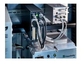
inspECT-PRO: Broadband multi-channel multi-frequency eddy current inspection electronics for multiple applications; inspection of weakly electrically conductive materials such as carbon fibers (CFRP)
