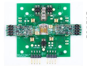
In electromobility, many small, efficient systems need to be integrated in limited space. The voltage converter shown is based on GaN power ICs measuring 4 x 3 mm<sup>2</sup>. © Fraunhofer IAF
