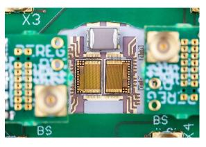
GaN power ICs with integrated transistors, gate drivers, diodes and current and temperature sensors for condition monitoring. © Fraunhofer IAF
