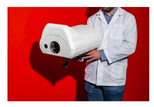
The hand-held scanner for hazardous substances identifies explosive, toxic and other hazardous substances in real time and shall help emergency personnel with on-site detections. © M-Squared Lasers PRESS RELEASE June 03, 2019 || Page 3 | 3
