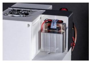
The core of the system is an extremely fast tunable quantum cascade laser with emission wavelengths in the mid-infrared range and high scan frequencies of up to 1 kHz. © Fraunhofer IAF
