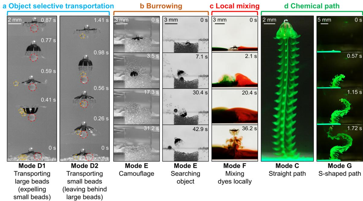
Figure 2. Four functions realized by the Jellyfishbot: a) transporting small and large beads; b) burrowing in a pool of fine beads simulating camouflage and search for prey; c) mixing two different colored food dyes; d) generating a chemical path.
