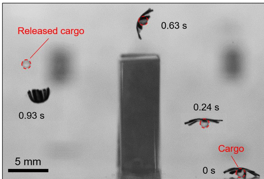
Figure 3. Cargo transport demonstration of the Jellyfishbot: The video snapshots of the robot and the bead are overlaid in the same video image. The red dashed circles indicate the positions of the bead being trapped and transported by the robot over a barrier.
