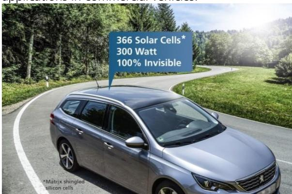
The MorphoColor® glass coating makes it possible to match the solar module's color to that of the vehicle.
